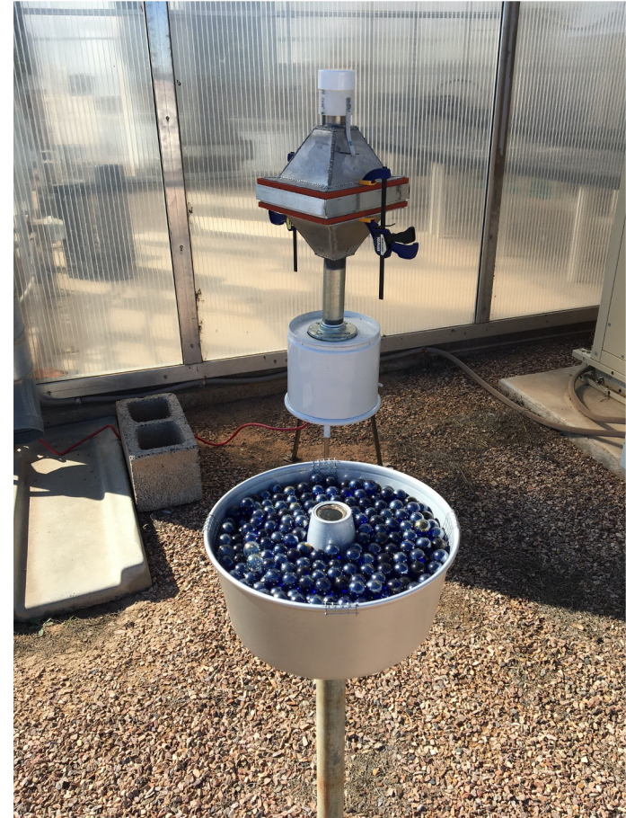
Installed Marble Collector (near) and Aspirated Sampler (far).
