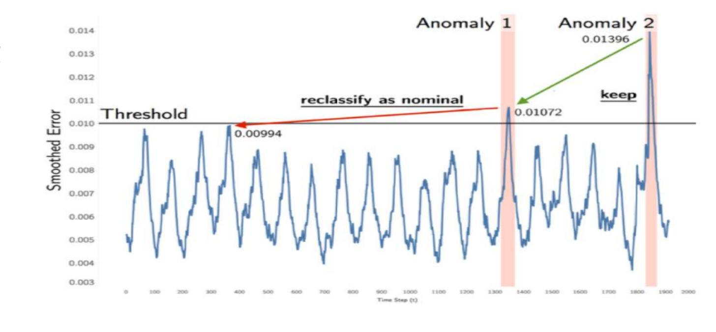
A threshold is found that, if all values above are removed, would cause the greatest percent decrease in the mean and standard deviation of the smoothed error.
