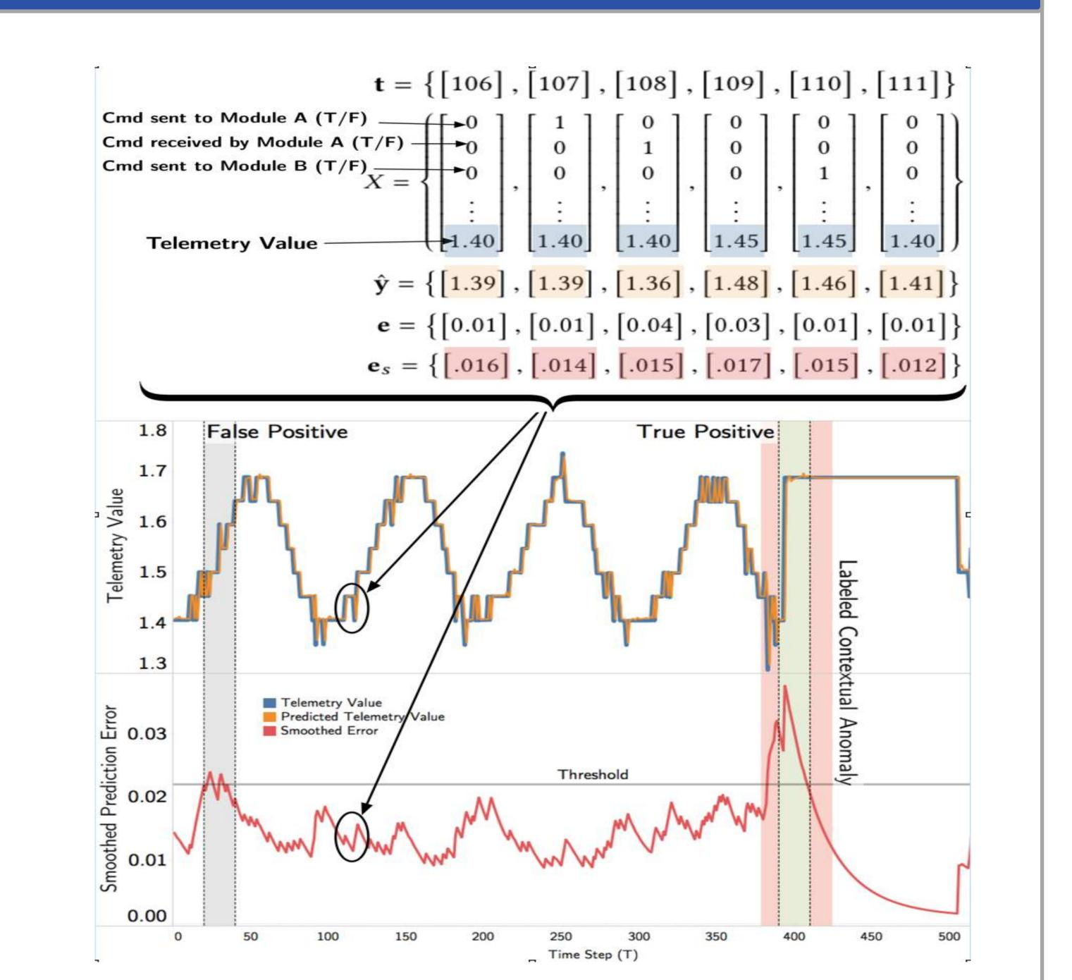
Smoothed errors  $\mathbf{e}_s = [e_s^{(t-h)}, \dots, e_s^{(t-l_s)}, \dots, e_s^{(t-1)}, e_s^{(t)}]$  A threst candidate thresholds  $\epsilon = \mu(\mathbf{e}_s) + \mathbf{z}\sigma(\mathbf{e}_s)$  above a greatest Threshold  $\epsilon = argmax(\epsilon) = \frac{\Delta\mu(\mathbf{e}_s)/\mu(\mathbf{e}_s) + (\Delta\sigma(\mathbf{e}_s)/\sigma(\mathbf{e}_s)}{n(\mathbf{e}_a) + n(\mathbf{E}_{seq})^2}$  mean a smooth smooth
