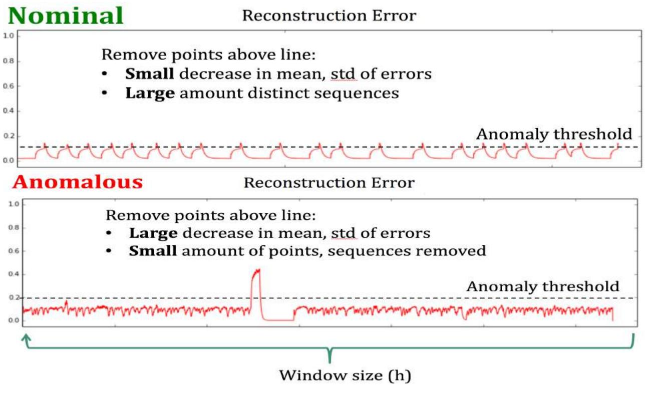
Pruning procedure (outlined in [1]) helps mitigate false positives, limit memory and compute cost, and ensure anomalous sequences are not the result of regular noise within a stream.
