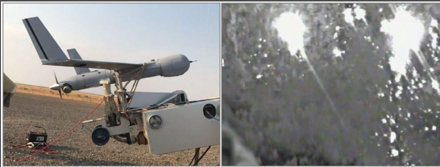
The Insitu Scan Eagle (above left) was one of four CWN awarded aircraft to fly in support of interagency wildfire operations in the summer of 2018. Overall, 86 flights were conducted on 16 different fires for more than 382 flight hours. Infrared sensors effectively identify “hot spots” (above right) with accurate geolocation data that is quickly relayed to firefighters on the ground (photo credit, Insitu (left) National Interagency Fire Center (right)).
