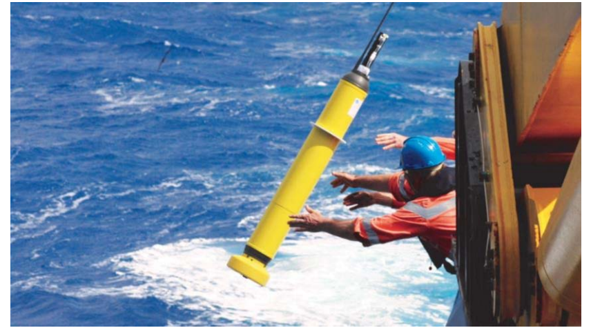
Argo floats are used to observe the ocean [image from Commonwealth Scientific and Industrial Research Organization]
