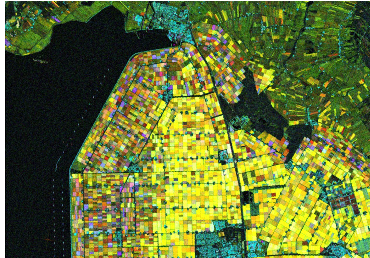
Sentinel-1 color composite (blue: mean of the July coherence; green: mean of the March coherence; red: seasonal standard deviation)
