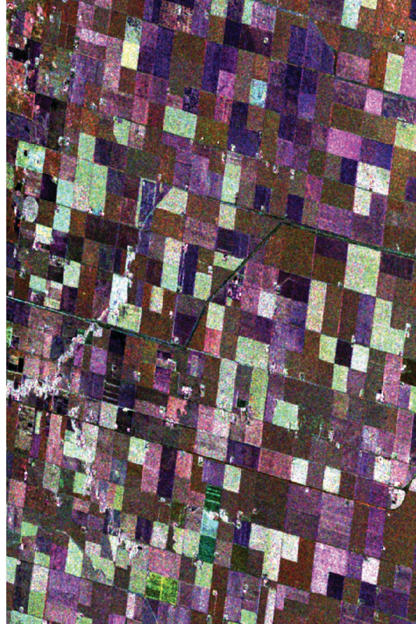
RADARSAT-2 (acquired on July 3, 2016, FQ15W). Slant range image (R: HH G: HV B:VV), in which distances are measured between the antenna and the target.
