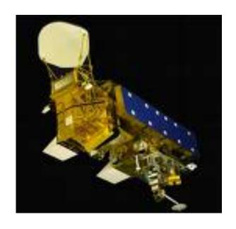
36 wavelength bands covering the wavelength range of 405 nm (blue) to 14.385 µm (infrared)
